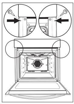
Then open the oven door and screw the oven to the side panels of the base unit through the two holes, one on each side of the oven trim.
